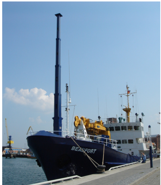
After retrofitting with extended telescopic mast for large SkySails systems
