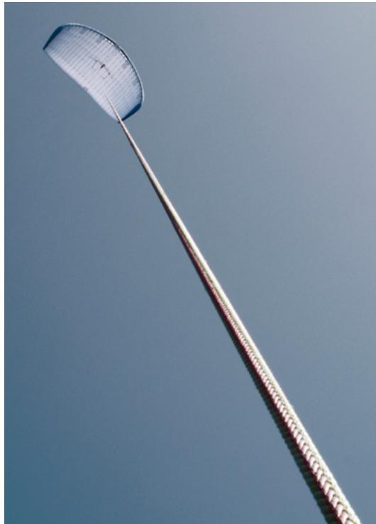
SkySails high performance towing rope made with Dyneema<sup>®</sup> and manufactured by Gleistein.
